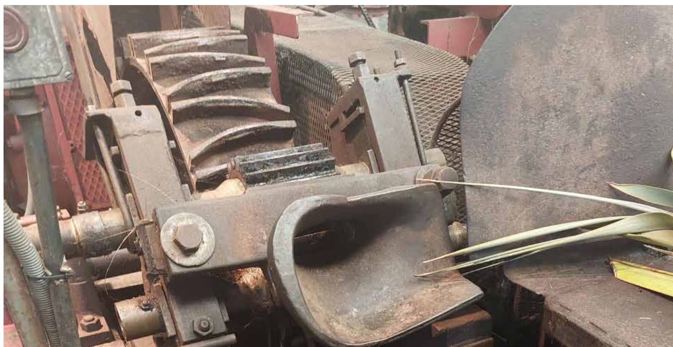
The flax stripping machines at Foxton, one of only two in the country and the only one still working.
